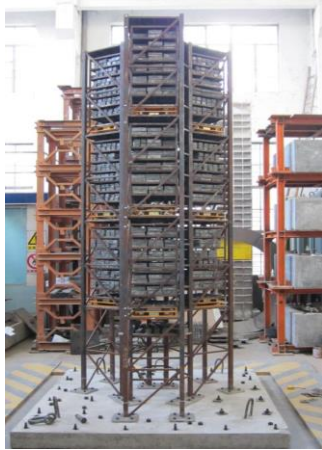
Vibration Table Test of the Seismic Mitigation and Control of the Giant Substructure
