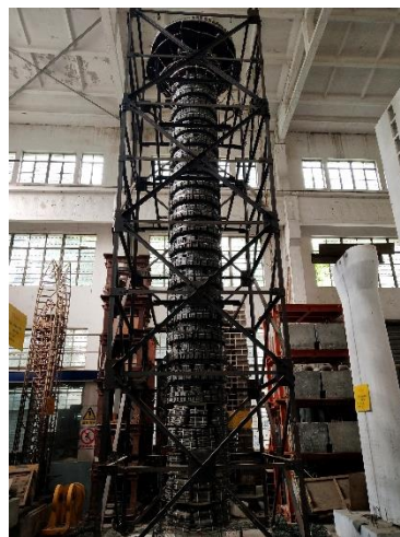
Shaking table test of Zhaoqing Landscape Tower
